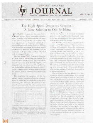
Fig. 5. (a) Jan. 1951. This issue describes the HP 524A High-Speed Frequency Counter. The counter provided frequency measurement up to 10 MHz and five selectable sampling periods: 0.001, 0.01, 0.1, 1.0, and 10.0 seconds. (b) July 1975. The HP 5328A Universal Counter has a direct count frequency range of 100 MHz (512 MHz with a special option), a period resolution of 100 ns (10 ns with a special module), and other functions such as time interval averaging, totalize, ratio, and so on. The HP Journal cover shows the counter's optional modules superimposed on a background showing the counter's interior. (c) Feb. 1989. The latest contribution to frequency and time measurement, the HP 5371A Frequency and Time Interval Analyzer. The cover shows a sculpture in plastic of the circuit diagram of a zero-dead-time counter, a key component in the HP 5371A. The HP 5371A uses a method known as continuous measurement technology. The zero-dead-time counters implemented with high-speed integrated circuits make one measurement after another without stopping. Like the HP 524A, this instrument has also made it easier to make certain frequency and timing measurements that were formerly difficult or impossible.
