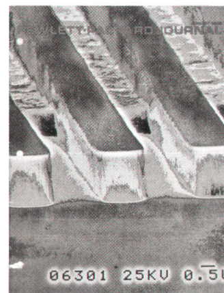
Fig. 13. Aug. 1982. The cover shows a solarized version of the profile of a trilayer process after reactive ion etching of the bottom polymer layer. This issue describes HP current and future efforts in integrated circuit process technology, particularly in the area of very large-scale integration (VLSI).
